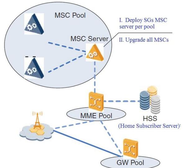
Fig.1. Options for deployment of CSFB
