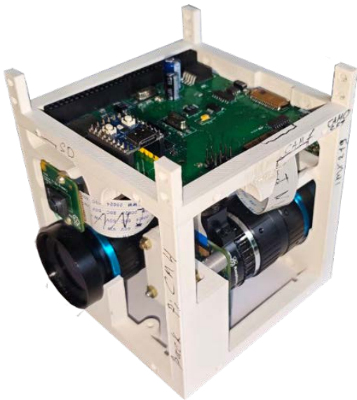
Figure 1. Experimental prototype of the EO-NANO module with 3D printing housing elements and four cameras
